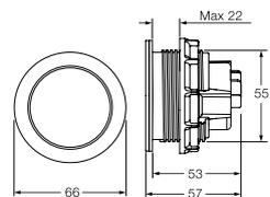
Always install some type of inspection hatch to access the valves in the cistern when selecting the pneumatic flush button
