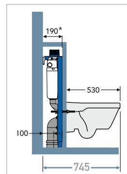
\*) The example presents the dimensions where the centre of the drain is 100 mm from the wall.
