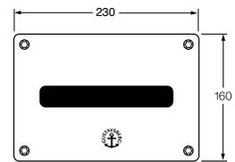
Sensor-controlled panel designed for public settings has different dimensions to other wall-mounted panels.
